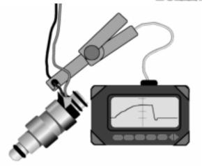
If you are working on a throttle body injected vehicle with the complaint of poor mileage, after checking all the basics, be sure to view the injector waveforms. If ringing is present install a 0.1 microfarad capacitor across the injector terminals. This should cure the problem.
