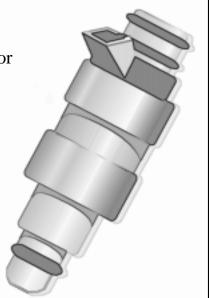
Whenever we suspect that we have a problem with the injectors, we should try to view their amperage waveforms. It will be easier to find opens and shorts using this method.
