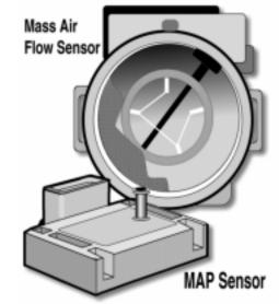
tion, however, since the leak allows air to enter the engine that the **air flow** sensor does not measure. If the air flow sensor doesn't detect the air flow, it won't request more fuel.
