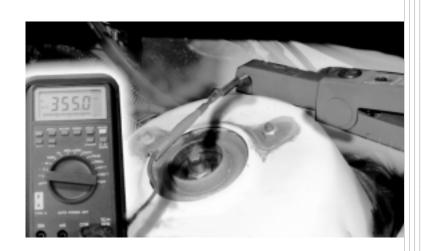
The maximum fuel pump current draw for CPI injected fuel pumps is 8-9 amps.
